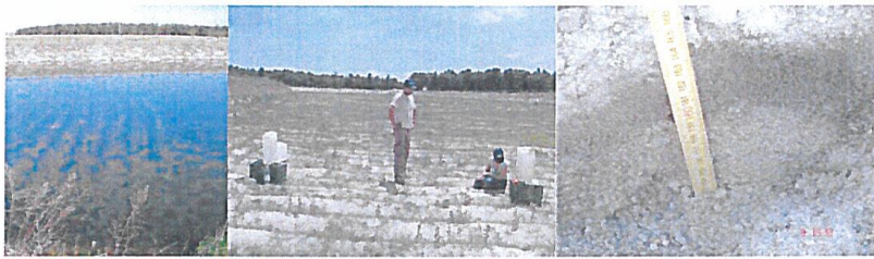
Figure 10. Furrows ploughed with different width at the bottom of a decantation and infiltration pond, infiltration test by double ring infiltrometer in the convex and concave surface of them and the clogging profile. Headwater of the Santiuste' AR device
