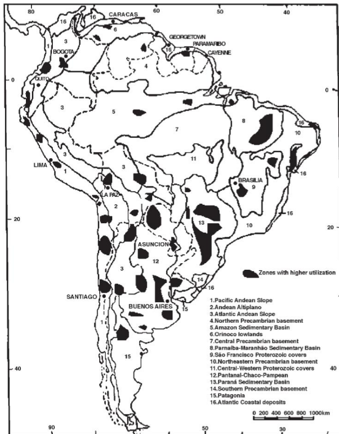
Figure 2-13: South America — Hydrogeological provinces and zones with higher utilization of groundwater. Illustration from Groundwater resources in South America (Rebouças, 1999). For an enlarge version of this image click here or scan the QR code.
