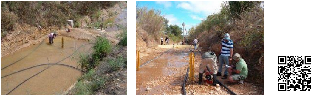
Figure 5-5: Rio Seco riverbed infiltration ponds (left image) and MAR clogging and infiltration experiments developed in Rio Seco (right image) (Campina de Faro, Algarve, Portugal). Illustrations from MARSOL. For more details on this MARSOL project click here or scan the QR code.
