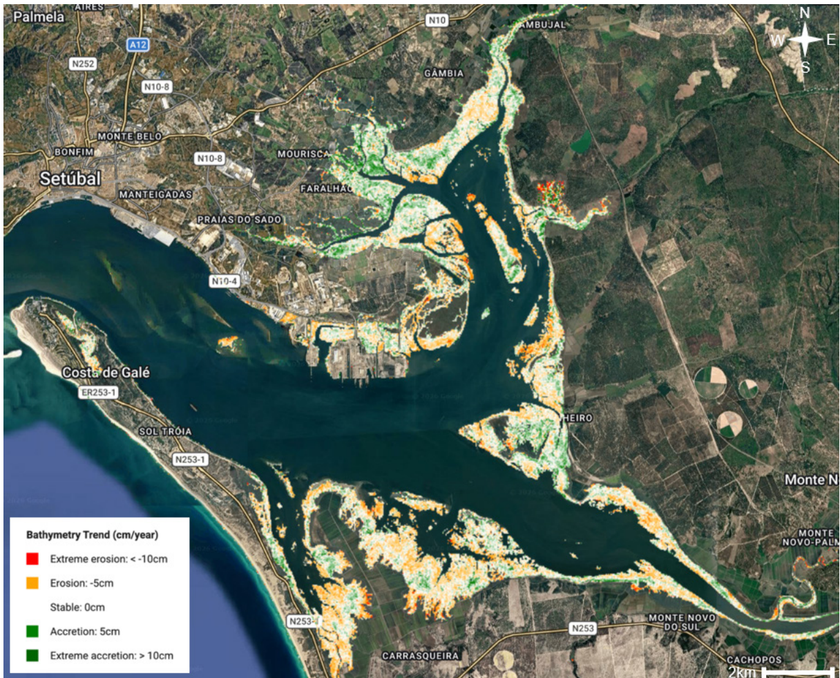
Figure 1- Erosion trend estimated over the last nine years (2017-2025) in the Sado estuary intertidal area. Green color indicates accretion, red indicates erosion and white indicates stability over the respective period.
