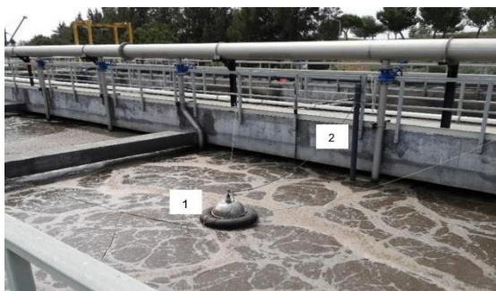
Figure 1 – Off-gas tool (1) and sensors for liquid phase measurements (2)
