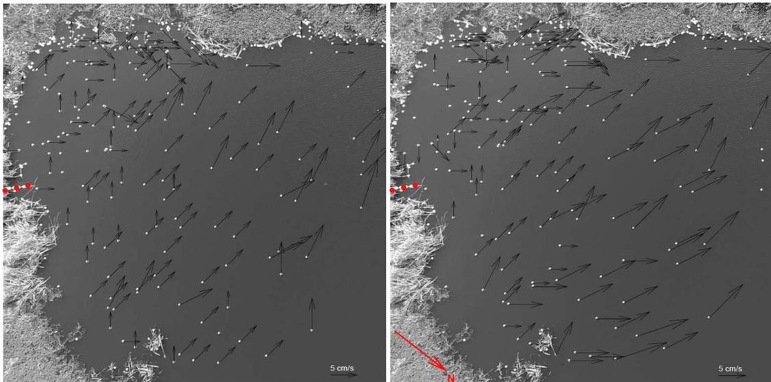
Fig. 3. Vector map of the free surface velocity of the Lake Vela at time instants 13:57:21.63 (left) and 13:57:33.30 (right).
