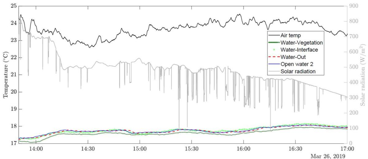
Fig. 2. Air and water temperature (left axis) and the solar radiation (right axis) acquired with the weather station and the temperature sensors.
