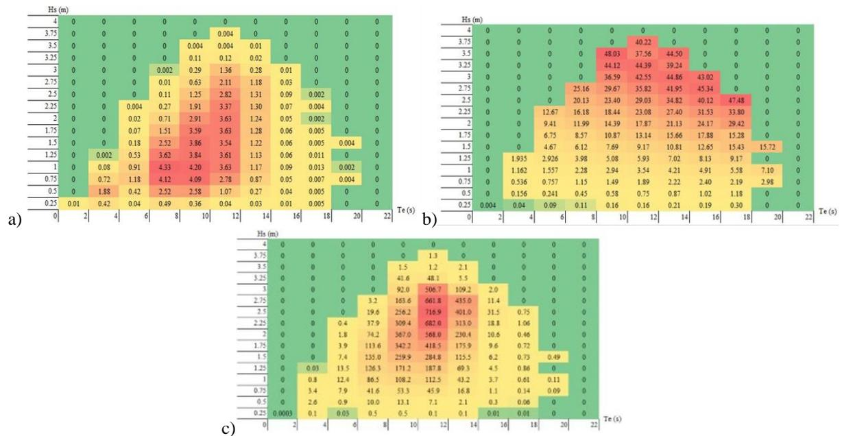
Fig. 2. Madalena do Pico: a) Occurrence frequency diagram for each sea state over the 40-year study period; b) Mean exploitable energy flux per wave front length in kW/m for each sea state over the 40-year of study; c) Combined occurrences and energy diagram multiplied by 8766h. Each bin indicates the value of the mean exploitable energy flux per wave front length ( $MWm^{-1}year^{-1}$ ).
